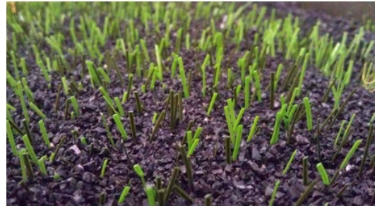
Tire crumb covering the plastic turf base
