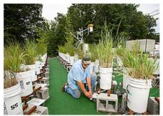
In simulated rain garden trials, technician Gary Lambert collects leachate to identify plants best able to slow movement of water, nutrients, and fecal bacteria through soil. (D1974-2)
