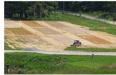
Subsoil compaction plots before topsoil is added. The red/orange subsoil is a Greenbrier County (West Virginia) limestone-based soil. The lightest colored plots are Raleigh County (West Virginia) sandstone, and the darker subsoils are Raleigh County shale.
