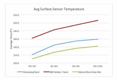
Surface Result: After 3.5 hrs. of controlled heat, Greenplay was found to be 47°f cooler than SBR rubber and within 20°f of natural grass.
