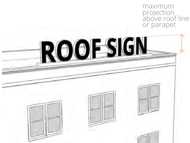
Figure 8.8-B Example of Roof Sign
