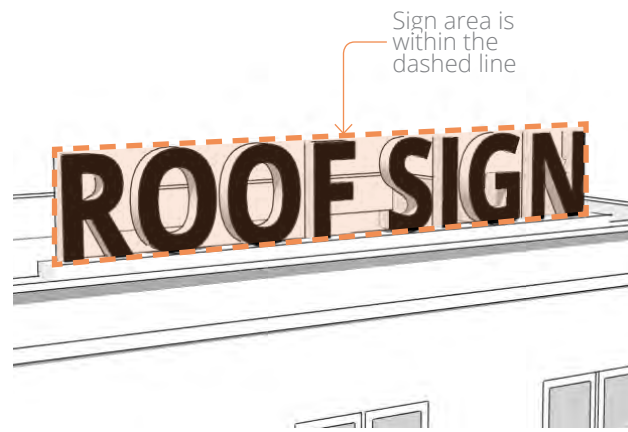
Figure 8.8-C Area Calculation for Roof Sign
