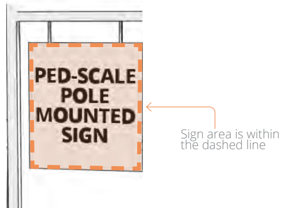
Figure 8.11-B Area Calculation for Ped-Scale Pole-Mounted Sign
