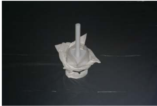
Figure 3: Weight with 1-quart polyethylene storage bag, a wipe (please note this is a paper towel for demonstration purposes only), and a cable tie
