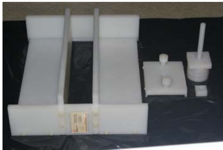
Figure 2: Sampling device frame, slide, weight and nut
